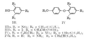
On hydrogenation of IVa three reactions, removal of the benzyl group, reduction of the nitro groups, and hydrogenation of the double bond in the side chain, were carried out in a single operation. Protection of the phenolic hydroxyl through the benzyl rather than the methyl ether may be advantageous in the synthesis of analogs of thyroxine other than the ones described in this paper, since a separate step for the removal of the protective group is avoided.
